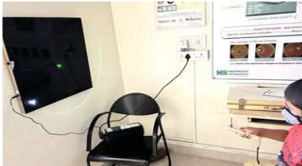
Figure 7: Photograph of orthoptek instrument. It has three rows of LEDs of white and central one is red
