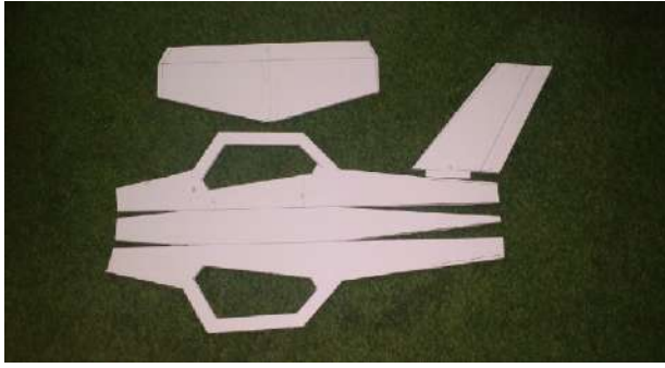
Figure 2 : The fuselage and the horizontal and vertical stabilizers of the Dragonfly were cut out from foam board which is light weight yet strong and durable. Carbon fiber rods are used to fortify the wing and fuselage. Traditionally Balsa wood is used to make model planes. But nowadays inexpensive and easily available foam sheets are the preferred building materials.
