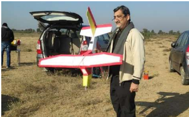
Figure 3 : Sanjivino stands proudly with the Dragonfly minutes before its maiden flight. The Dragonfly has a wing span of 1.4 meters and a total weight of 900 grams. The motor is a 1400KV rating brushless one and the transmitter and receiver are of Futaba make. The plane is a “high wing” type, meaning the wings sit on top of the cockpit. This wing placement and its under camber [hollow curve] give the plane stability and slow fly characteristics.
